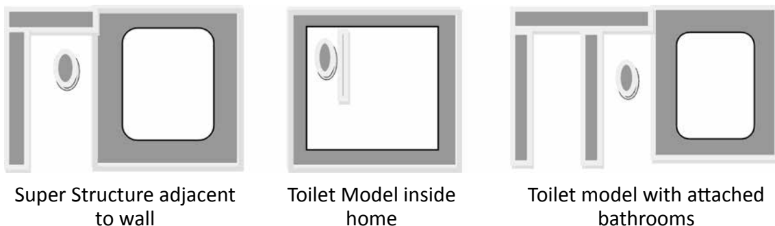
Figure 15: Models for Superstructure of Toilets
